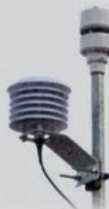
The DOL 58 weather station allows including the local weather conditions in the ventilation control. Wind direction, air speed and air pressure are measured for this purpose.
