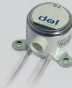
DOL 18 is a negative-pressure sensor that actively measures the pressure in the barn, emitting a 0-10 V signal. The climate computer usually supplies the sensor with a voltage of 15 to 30 V DC.
