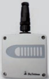
DOL 19 measures the house air's carbon dioxide content. Its high-quality infrared measuring cell is able to detect CO<sub>2</sub> in a range from 0 to 10,000 ppm. It is thus possible to control minimum ventilation based on the CO<sub>2</sub> concentration. This saves heating costs and makes for an improved house climate.
